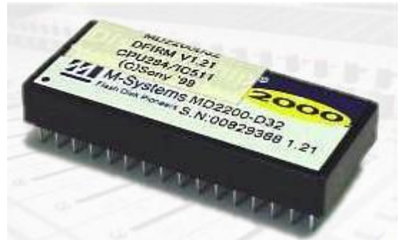
(Fig 2) Disk-on-Chip 2000 (Earlier Units)
